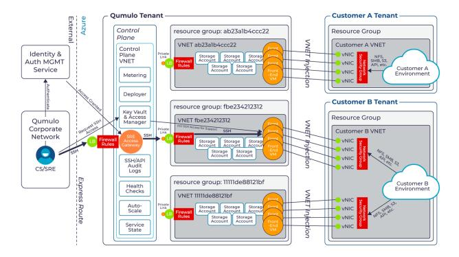
The Qumulo architecture separates the control plane from the data plane.
